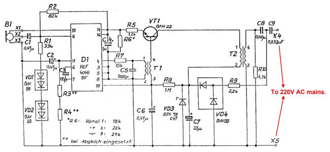
Circuit diagram of a TF-B tx (2A) bug 33603-101...103 or 111...113
